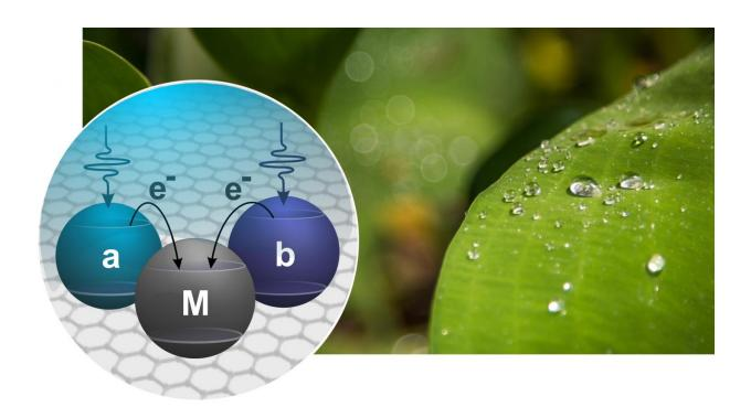
In a light harvesting quantum photocell, particles of light (photons) can efficiently generate electrons. When two absorbing channels are used, solar power entering the system through the two absorbers (a and b) efficiently generates power in the machine (M). Credit: Nathaniel Gabor and Tamar Melen
