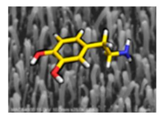
Image of carbon nanofibre surface with a modelled dopamine molecule on top, taken with a scanning electronic microscope. Credit: University of Helsinki
