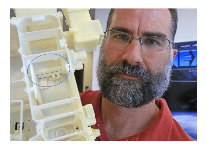
SwRI's Dr. Thomas Greathouse uses an engineering model of the Lyman-Alpha Mapping Project (LAMP) instrument to show a failsafe door (outlined by rectangle) recently opened in lunar orbit. Located below the regular aperture door (circled), the door opened flawlessly, even after orbiting the moon for seven years onboard NASA's Lunar Reconnaissance Orbiter (LRO), providing LAMP more UV exposure for LRO's extended mission. Credit: Southwest Research Institute
