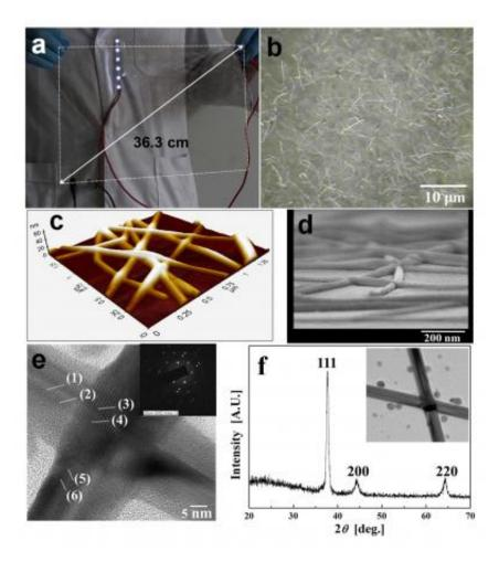
Left, photograph of a large-scale silver nanowire-coated flexible film. Right, silver nanowire particles viewed under the microscope. Credit: S.K. Yoon, Korea University
