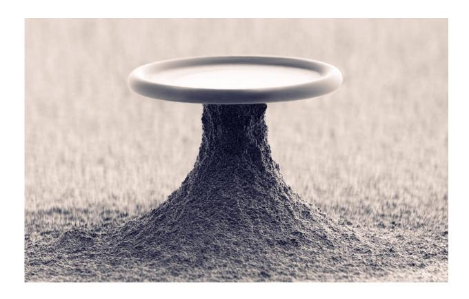
SEM micrograph of a microtoroidal resonator similar to the one used for demonstration of quantum-enhanced feedback cooling. The silica torus forms a cavity for light which is modulated by the mechanical vibrations of the supporting disk. Light is coupled in and out of the system by bringing a tapered optical fiber in proximity of the torus. Credit: Kristian Rasmussen, DTU
