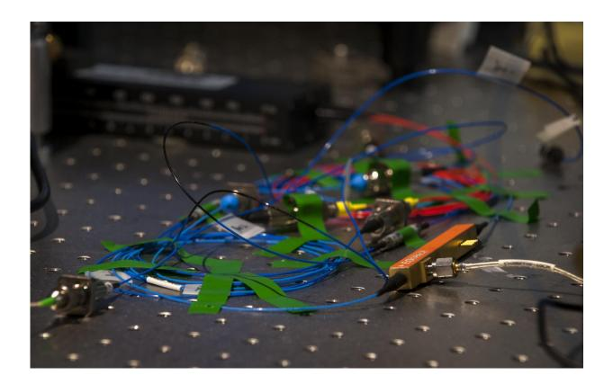
A single photon converter (a yellow-orange box) installed on an optical fiber of the laboratory setup. Credit: UW, Grzegorz Krzysewski
