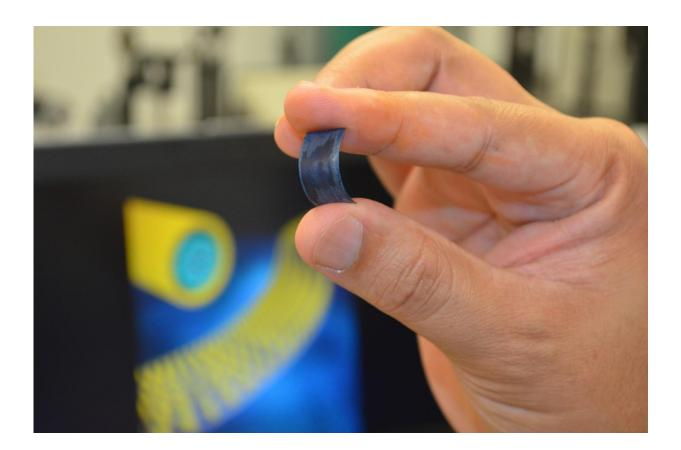
A thin, flexible supercapacitor developed at the University of Central Florida boasts high energy and power densities. Credit: University of Central Florida
