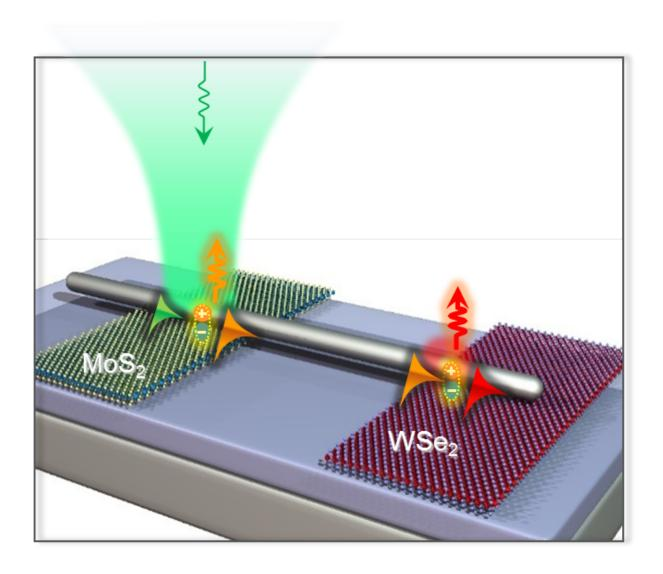
The multiplexer device with one input and two outputs. The plus-minus couple indicates the exciton. Credit: Institute for Basic Science
