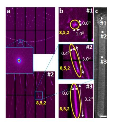
This image shows the results of scanning X-ray microdiffraction ( $\mu SXRD$ ) with submicron spatial resolution. Lauediffraction (a) from an unconstrained Sb2S3 single crystal (top) and laser fabricated RLS crystal Sb2S3 (bottom). Magnified images (b) of selected reflection (852) extracted from Laue patterns (a, bottom) obtained for differentpoints of the RLS crystal (c). Credit: D. Savytskii, H. Jain, N. Tamura & V. Dierolf
