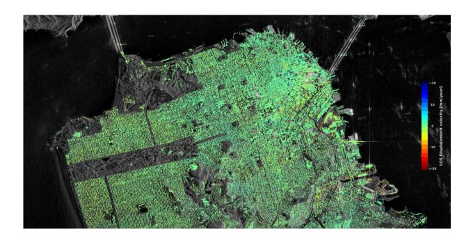
Sentinel-1 radar data show ground displacement of downtown San Francisco. While green indicates no detected movement, points in yellow, orange and red indicate where structures are subsiding, or sinking. Credit: Contains modified Copernicus Sentinel data (2015–16) / ESA SEOM INSARAP study / PPO.labs / Norut / NGU
