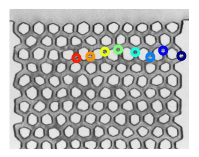
Rigid materials break in straight narrow patterns, as shown by the line of colored dots where this piece of plastic lattice failed. Credit: Prof. Sidney Nagel, et al.
