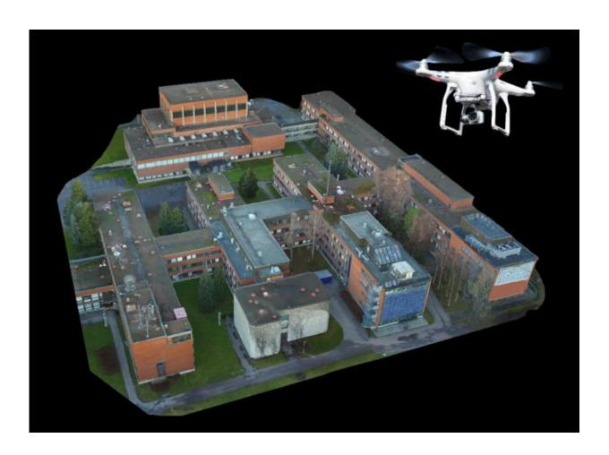
By using both the aerial photographs taken by the drone and photogrammetry software, researchers were able to create highly detailed 3-D models of urban environments. Credit: Vasilii Semkin / Aalto University
