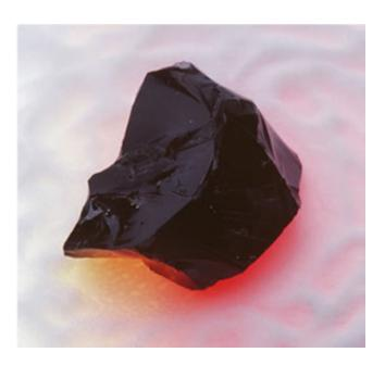
Glass produced from a high level radioactive waste simulant. Credit: Albert Kruger/U.S. Department of Energy
