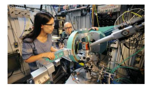
Caltech graduate student Yishu Wang and Argonne scientist Yejun Feng are working at the research station of the Argonne National Lab/APS. The experimental setup is for doing magnetic diffraction at low temperature and high pressure. Credit: Argonne National Laboratory/APS
