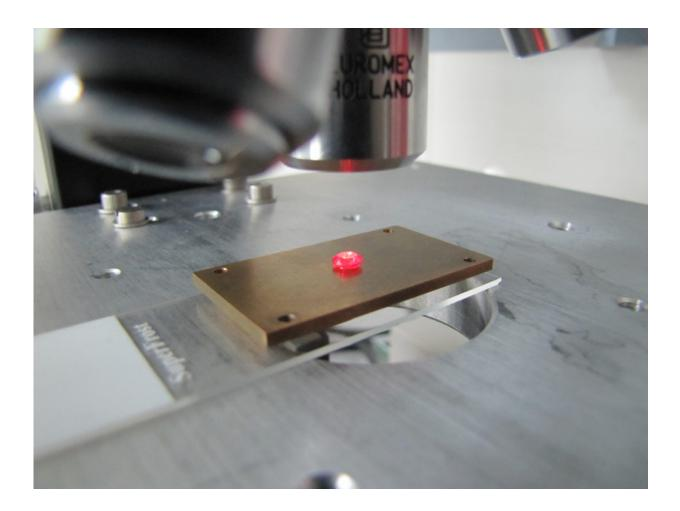
An artificial diamond under the optical microscope. The diamond fluoresces because due to a number of nitrogen defects. Credit: Vienna University of Technology
