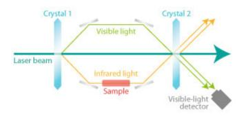
By creating an entangled pair of one infrared photon and one visible light photon, A\*STAR researchers can perform infrared measurements on a sample by detecting only the visible light photon. Credit: *Nature Communications* (Ref 2), copyright (2016)
