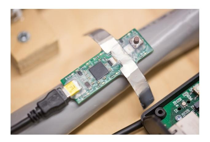
With support from the Office of Naval Research (ONR), researchers at the Massachusetts Institute of Technology have designed a portable measurement system to precisely and cheaply monitor the amount of electricity used by individual household appliances, lighting fixtures and electronic devices. Credit: Bryce Vickmark
