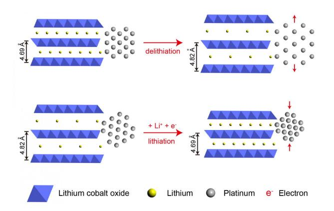
Bottom:Platinum atoms attached to layers of lithium cobalt oxide contract when electricity is applied, boosting platinum catalytic efficiency by 90 percent. Top: Removing electrons separates the atoms and lowers efficiency by 40 percent. (1?Ångstrom = 0.1 nanometer) Credit: Haotian Wang
