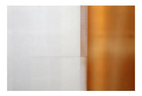
Streamwise-oriented 'finlets' are installed on a wing or blade trailing-edge to reduce trailing-edge noise by up to 10dB without substantial changes to the aerodynamic performance and over a range of angles of attack. Credit: Nathan Alexander
