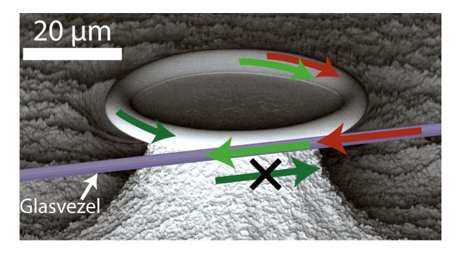
With the help of an optical fibre (purple), the researchers were able to trap light in a ring. When two different colours (red and light green) start to circulate in the same direction in the ring, then the ring starts to vibrate. As a result of this, light is allowed to pass through. As the dark green light moving in the opposite direction does not cause the ring to vibrate, light in that direction is blocked. Credit: Fundamental Research on Matter (FOM)
