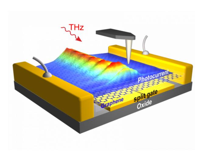
THz plasmons of extremely short wavelength propagate along the graphene sheet of a THz detector, as visualized with photocurrent images obtained by scanning probe microscopy. Credit: Nature Nanotechnology
