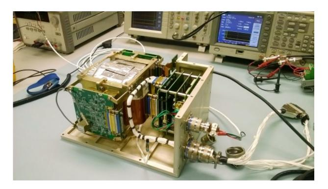
The Fast Neutron Spectrometer with a cover removed to show the circuitry inside. Credit: UAH
