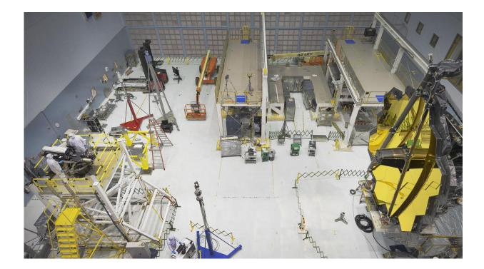
Engineers conduct a 'Center of Curvature' test on NASA's James Webb Space Telescope in the clean room at NASA's Goddard Space Flight Center, Greenbelt, Maryland. Credit: NASA/Chris Gunn
