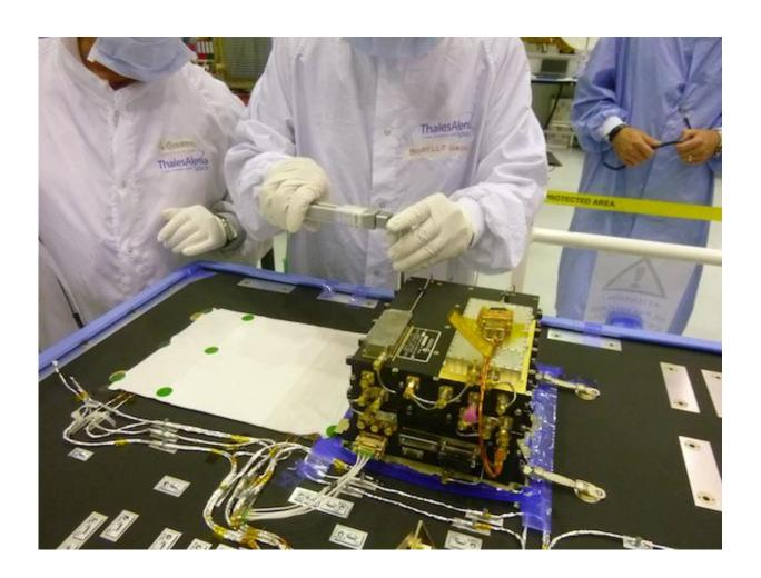
The European Space Agency's ExoMars Trace Gas Orbiter, launched on March 14, 2016, carries two Electra UHF relay radios provided by NASA. This image shows a step in installation and testing of one of those radios, inside a clean room at Thales Alenia Space, in Cannes, France, in June 2014. Credit: NASA/JPL-Caltech/ESA/TAS
