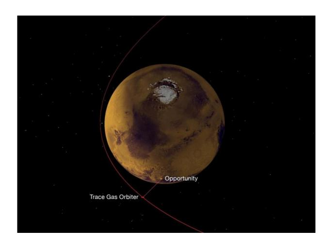
A NASA radio on Europe's Trace Gas Orbiter, which reached Mars in October 2016, has succeeded in its first test of receiving data from NASA Mars rovers, both Opportunity and Curiosity. This graphic depicts the geometry of the relay from Opportunity to the orbiter, which then sent the data to Earth. Credit: NASA
