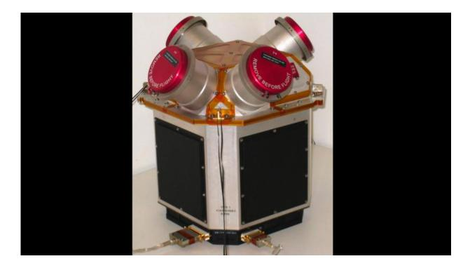
This cluster of four colloid thrusters, part of the Disturbance Reduction System developed by NASA/JPL, helps keep the LISA Pathfinder spacecraft extremely stable. Credit: NASA
