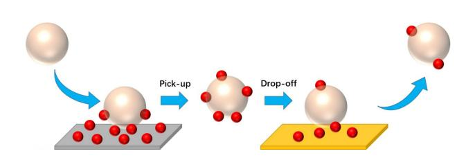
Oil-in-water droplets represented by shiny spheres stabilized by functional surfactants first pick up the nanoparticles, represented by small red balls, when traversing a nanoparticle-coated surface. Later in the same in-line process, when the particle-attached droplets meet the downstream empty surface with a high affinity for the nanoparticles, they drop the nanoparticles off onto the surface and move forward in the aqueous flow. Credit: UMass Amherst/Richard Bai
