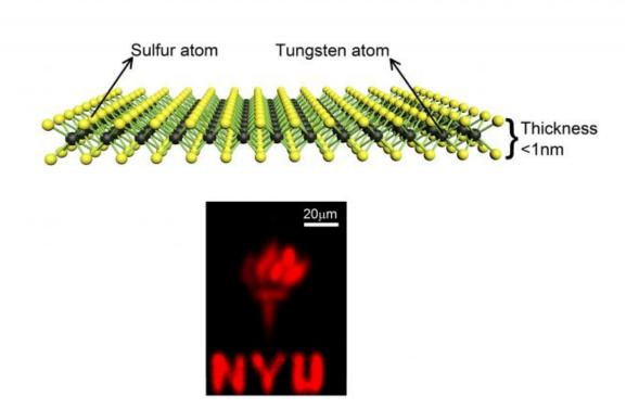
At just one atom thick, tungsten disulfide allows energy to switch off and on -important for nano-scale electronic transistors -- but it also absorbs and emits
