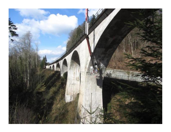
Detailed radar and ultrasonic measurements were made from a mobile platform underneath the Laufenmühle viaduct. Credit: IONYS/KIT
