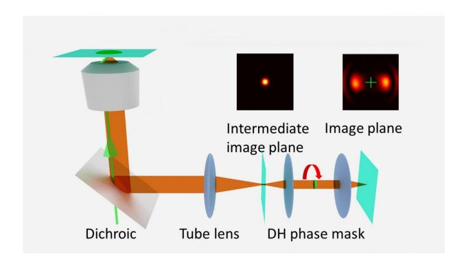
A schematic shows a Rice University technique called super temporal resolution microscopy, which acquires faster molecular movies without needing a faster camera. A spinning "double helix" phase mask turns the single-point image of a molecule into barbell-shaped lobes that change angle depending on the time the image is captured. A molecule may be captured multiple times in a single image. Credit: Landes Research Group/Rice University
