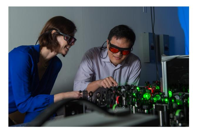
Rice University chemist Christy Landes, left, works with postdoctoral researcher Hao Shen to adjust lasers for the lab's super temporal resolution microscope. The lab invented a technique to acquire better data about molecules that move faster than a standard lab camera can capture. Credit: Jeff Fitlow/Rice University
