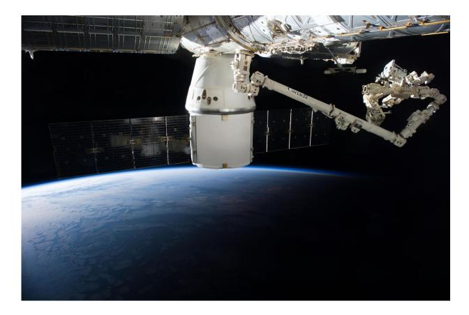
A view of the removal of the RapidScat Nadir Adapter from the SpaceX-4 Dragon trunk and installation of the adapter onto the Columbus Exposed Facility Unit (EFU).The RapidScat instrument was the first piece of technology to be robotically assembled in space since the station's construction, as well as the first scatterometer to be able to cross-calibrate with other instruments in orbit. Credit: NASA
