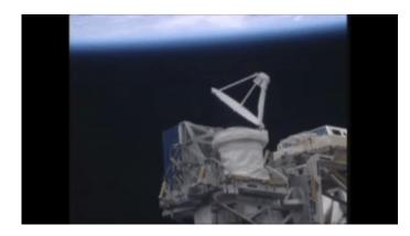
RapidScat's radar technology used microwaves, bounced off the ocean's surface, to determine wind speed and direction. Credit: NASA
