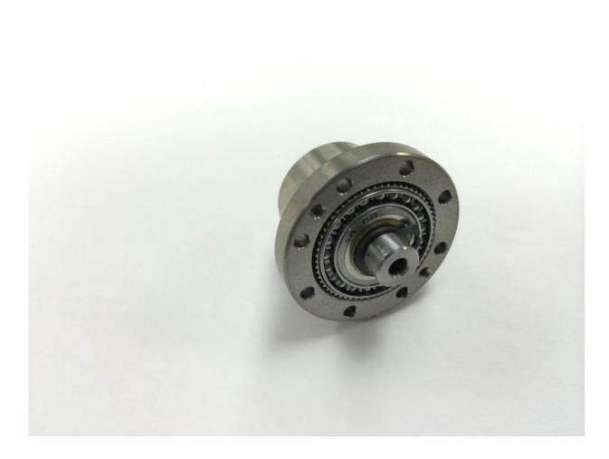
An example of a strain wave gear, also known as a harmonic drive - one of the most expensive types of gears used in high-precision robotics. As the gear turns, the flexible ring inside it squeezes, becoming an oval shape. Credit: NASA/JPL-Caltech
