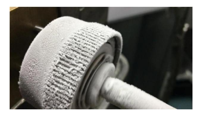
Bulk metallic glass, a metal alloy, doesn't get brittle in extreme cold. That makes the material perfect for robotics operated in space or on icy planets. Credit: NASA/JPL-Caltech
