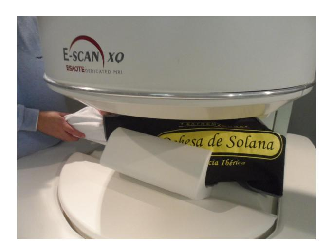
The University of Extremadura have developed a non-destructive, innocuous method using magnetic resonance, computer vision and statistical calculus that enables one to quantify the salt content of Iberian ham. Credit: UEx
