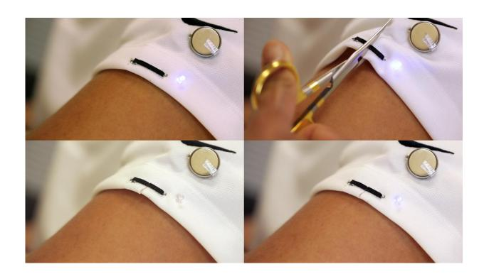
Nanoengineers printed a self-healing circuit on the sleeve of a T-shirt and connected it with an LED light and a coin battery. The researchers then cut the circuit and the fabric it was printed on. At that point, the LED turned off. But then within a few seconds it started turning back on as the two sides of the circuit came together again and healed themselves, restoring conductivity. Credit: Jacobs School of Engineering/UC San Diego
