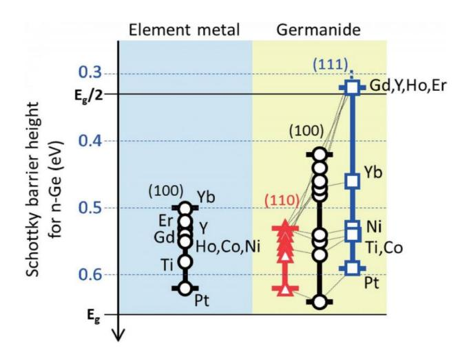
Experimentally obtained Schottky barrier height (SBH) at element metal/n-Ge and germanide/n-Ge interfaces. By designing the metal and interface structure of Ge, the SBH at the direct metal/n-Ge interface is controllable to be less than half of the band gap of Ge. Credit: Japan Society of Applied Physics (JSAP)
