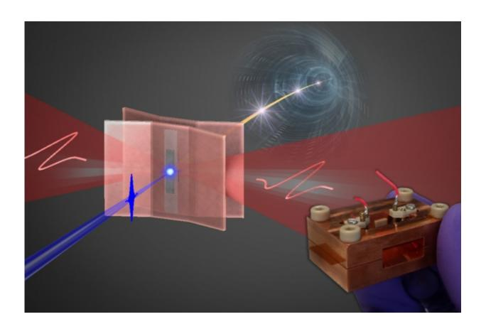
This illustration shows a miniature electron gun driven by terahertz radiation. A UV pulse (blue) back-illuminates the gun photocathode, producing a high-density electron bunch inside the gun. The bunch is immediately accelerated by ultra-intense terahertz pulses to energies approaching 1 kiloelectronvolt. These high-field optically-driven electron guns can be utilized for ultrafast electron diffraction or injected into the accelerators for X-ray light sources. Credit: W.
