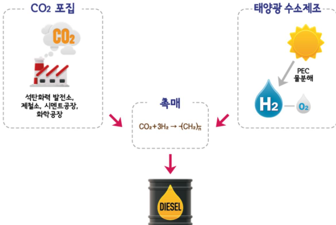
Proposed carbon capture and utilization (CCU) system based on catalytic CO<sub>2</sub> conversion to liquid hydrocarbon fuels with hydrogen supplied from solar water splitting. Credit: Ulsan National Institute of Science and Technology
