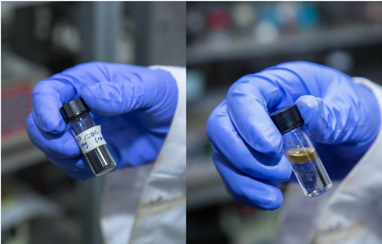
The sample on the left is the new delafossite-based catalyst used in the reaction between  $\text{CO}_2$  and  $\text{H}_2$  generated by solar water splitting. Shown on the right is diesel, produced by the reaction. Credit: UNIST
