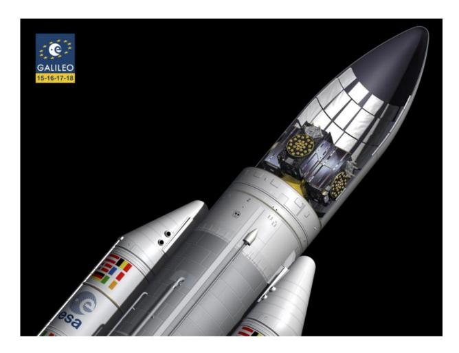
Cutaway view shows the four Galileo satellites mounted on top of a specially adapted Ariane 5 rocket underneath the aerodynamic fairing. Credit: ESA–P. Carril
