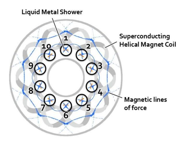
The magnetic field lines that confine a high-temperature plasma and the liquid metal shower divertors, as seen from above through a cross-section. Credit: Dr. Junichi Miyazawa
