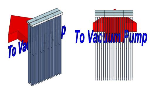
(left) The liquid metal shower functions as a shielding wall for plasma, (right) it is almost transparent for neutralized plasma. Credit: Dr. Junichi Miyazawa
