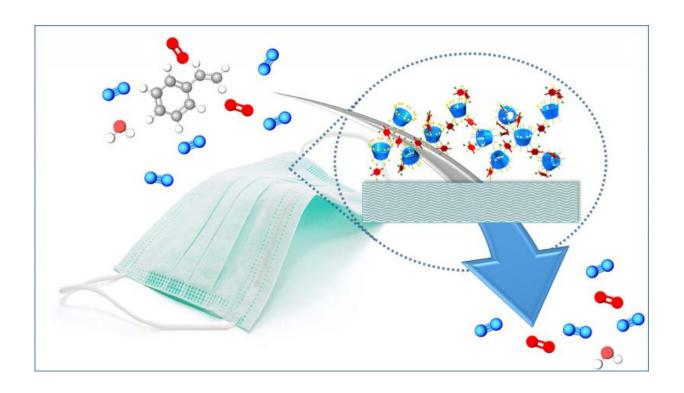
Cup-shaped beta-cyclodextrin polymers are infused into fabric during the polymerization process, giving the fabric the ability to sequester pollutants in both water and air. Credit: Juan Hinestroza/Provided
