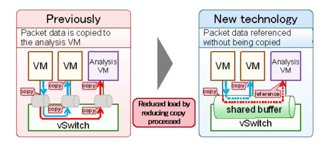
Figure 2: Load-reducing capture technology in virtual networks
