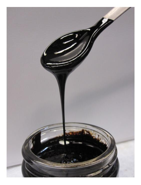
Biocrude oil, produced from wastewater treatment plant sludge, looks and performs virtually like fossil petroleum. Credit: WE&RF
