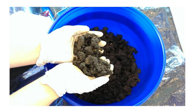
Sludge from Metro Vancouver's wastewater treatment plant has been dewatered prior to conversion to biocrude oil at Pacific Northwest National Laboratory. Credit: Courtesy of WE&RF
