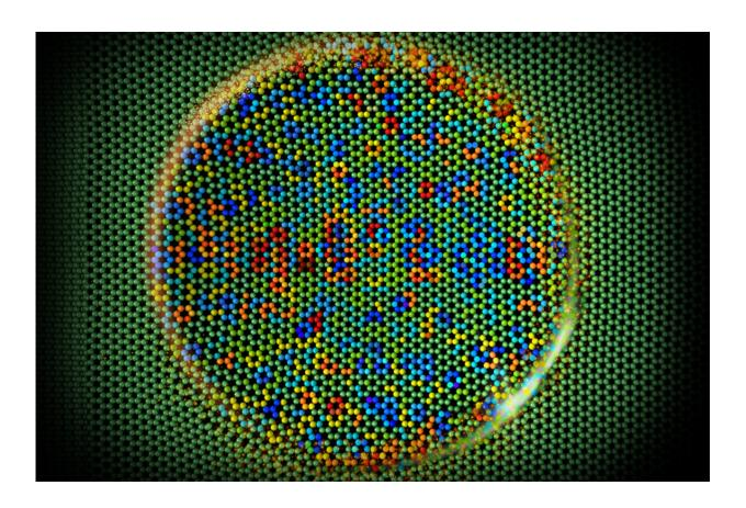
Images produced from computer simulations show the response of a graphene surface as a silicon tip slides over it. Relative forces of atomic friction on the surface are shown by colors: Red points are "pushing" sites that help propel the tip along the surface, while blue points are "pinning" sites of greater friction that inhibit the tip's motion. Credit: Courtesy of the researchers
