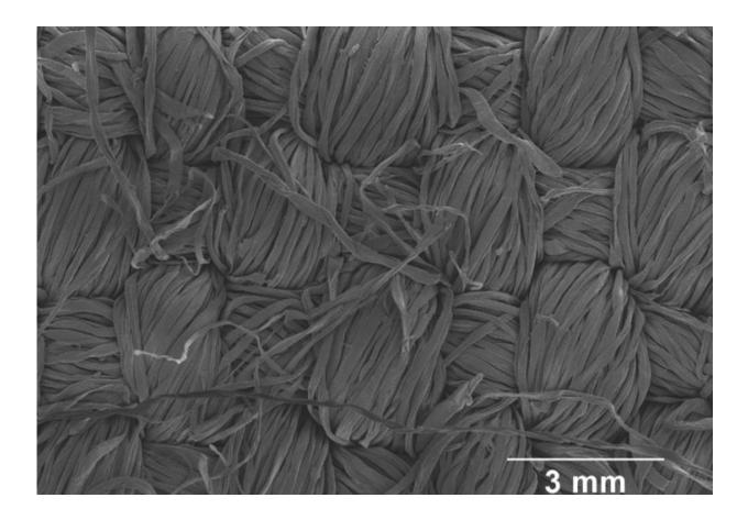
Electron microscopy image of a conductive graphene/cotton fabric. Credit: Jiesheng Ren
