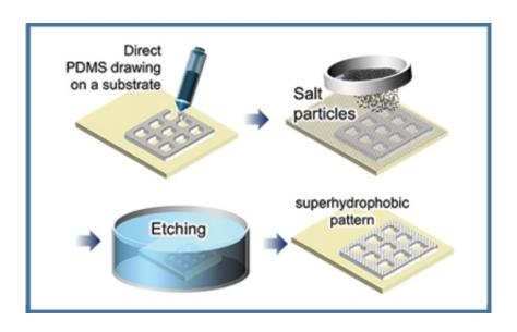
The POSTECH research team developed an innovative salt dissolution assisted etching method for facile and cost-effective fabrication of patternable superhydrophobic surfaces. Credit: POSTECH
