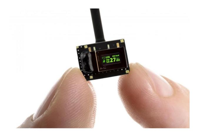
Fraunhofer researchers have developed an energy-saving display that reduces the power consumption to a fraction. Credit: Fraunhofer FEP
