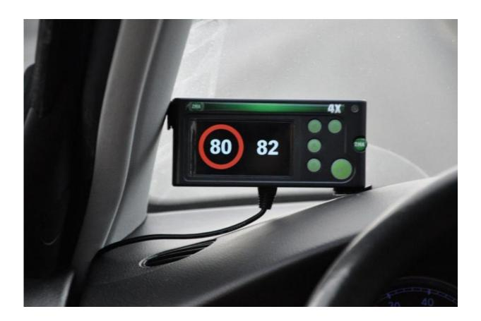
This is how the system appears to the driver. The 81 - 84 km/h range in an 80 km/h zone displays a flashing speed limit symbol. Beyond 84 km/h, an auditory signal is added to the flashing display. Credit: SINTEF
