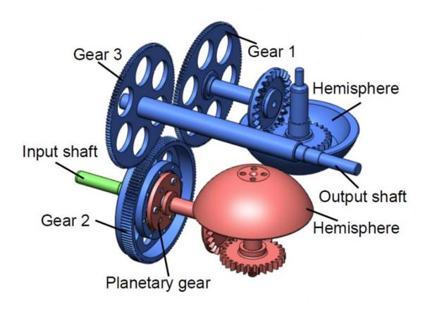
Dual-hemisphere continuously variable transmission (CVT). Credit: University of Twente
