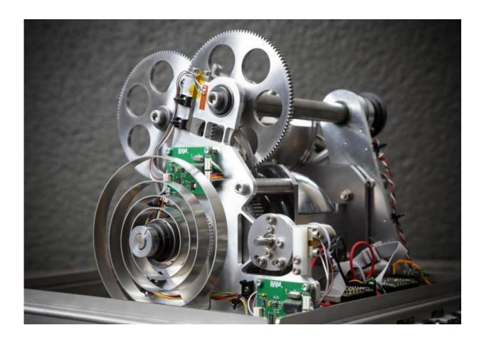
The robot's drive train including the dual-hemisphere system. Credit: University of Twente
