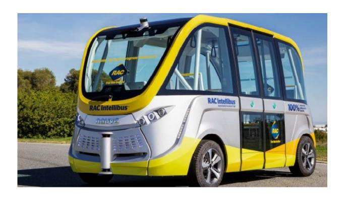
The RAC Intellibus<sup>TM</sup> is able to carry 11 passengers and reach speeds of 45 km/hr. Credit: RAC
