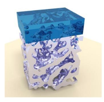
An illustration of the nanomaterial with alumina coating, based on a three
