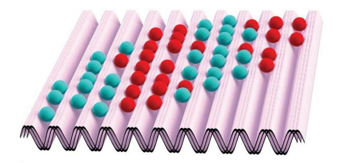
In an experiment at UChicago that witnessed a phase transition of quantum cesium atoms, an optical lattice lined the atoms up in patterns based on their positive or negative momentum. The lattice was shaken to drive the atoms across the phase transition and divide into different domains. Credit: University of Chicago
